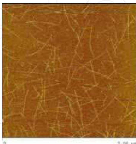
Fig. 7. Atomic force microscope image of synthesized imogolite.
