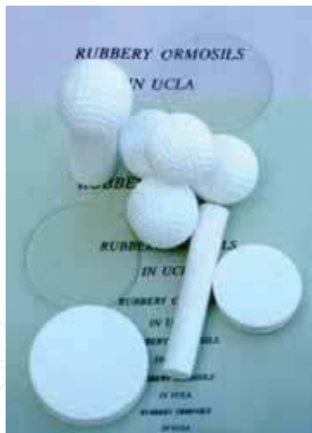
Fig. 13. Rubbery hybrids with different shapes (from Sanchez et al., 2005).
