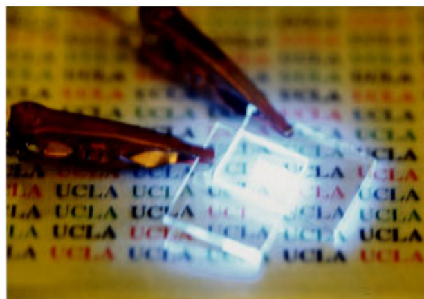
FIG. 5. Picture of a biased SLED, showing a strong blue electrochemiluminescence emission.
