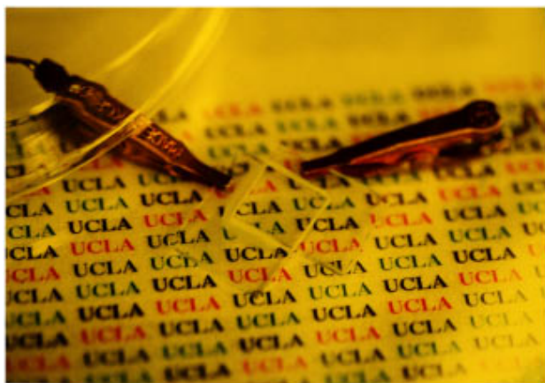
FIG. 4. Picture of an unbiased SLED, showing the transparent devices. The transmittance is higher than 90%.
