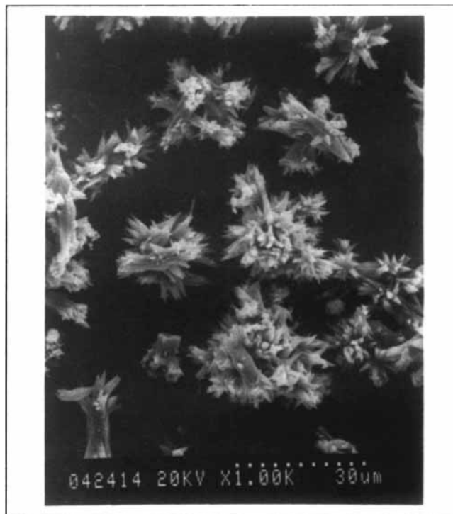
Figure 14. Rosette aragonite with 5 mM \text{Mg}^{2+} present in the solution.
