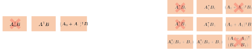
(a) 1D MDS-code [5] in an example with 3 workers that can each store half of A and the entire B .
