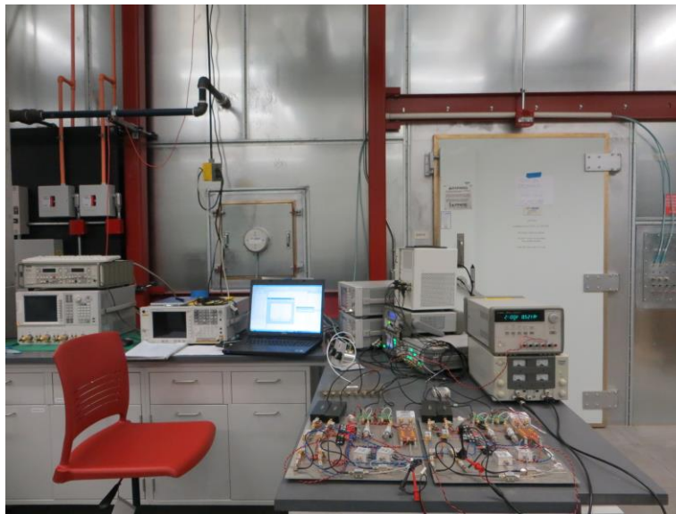
Figure 11: L-band radar test bed (anechoic chamber in background)
