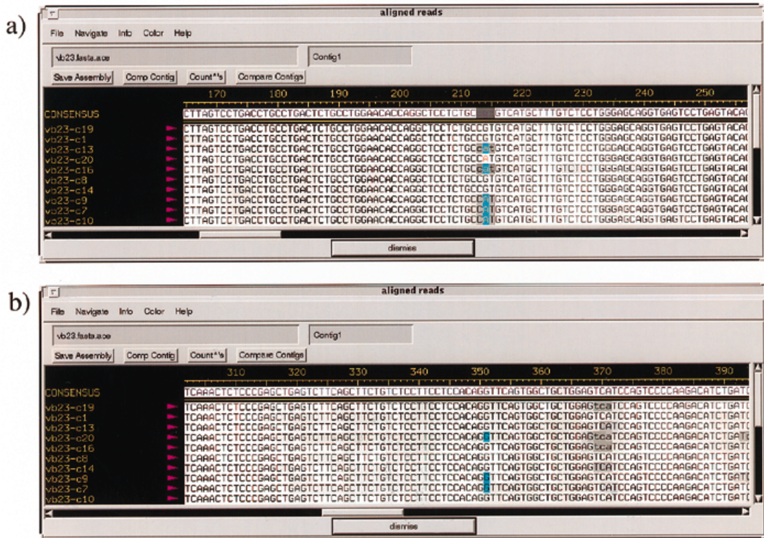
Figure 1. Two windows from the ‘color means quality and tags view’ of the Consed program. Sequences from two TCR \beta sites (in TCRVB23) obtained by dye-primer sequencing of PCR products from 10 different individuals are shown in each window. In Consed, sequence quality measured by Phred is depicted using a gray scale with a white background indicating the highest quality bases and increasing shades of gray indicating decreasing data quality. Potential heterozygotes identified by PolyPhred are color coded in blue in this Consed view. (a) When a common DNA polymorphism is identified (e.g. position 214) homozygotes for each of the alternative alleles and heterozygotes (highlighted blue) are normally detected. (b) Less common DNA variants usually appear as rare heterozygotes among a background of homozygotes (e.g. position 351). There are no false positives or false negatives identified in these windows and the genotypes of these individuals were completely consistent with those obtained by PCR/OLA.
