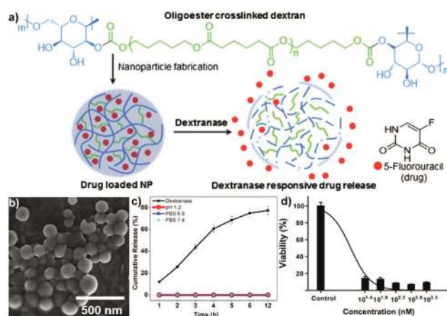
Fig. 10 (a) Schematic overview for nanoprecipitation assisted fabrication of DEXNPs in the presence of 5-FU, as well as depiction of dextranase responsive drug release, (b) SEM image of 5-FU loaded DEXNPs, (c) release kinetics of DEXNPs at simulated pH 1.2, PBS 6.8, PBS 7.4 & dextranase (15 U mL -1 ) and (d) cytotoxicity of DEXNPs against HCT 116 colon cancer cell line after 1 h of exposure of DEXNPs to dextranase. (Reproduced with permission from ref. 217. Copyright Elsevier, 2020.)
