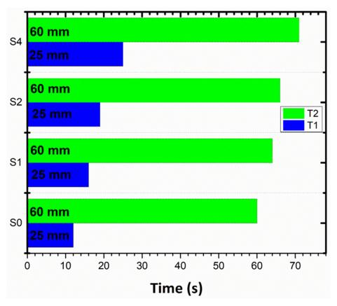
**Figure 10.** Increase in flame retardancy upon addition of m-sepiolite from S0–S4 samples in terms of T1 and T2.
