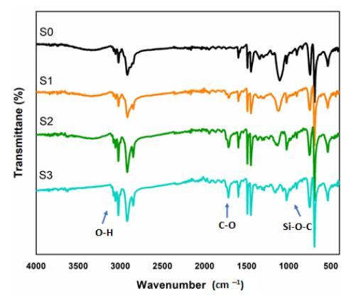
Figure 3. FTIR spectra of S0 (pristine PS), S1 (PS/1 wt.% m- sepiolite), S2 (PS/2 wt.% m-sepiolite) and S4 (PS/4 wt.% m-sepiolite).
