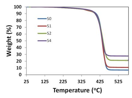
Figure 8. TGA analysis of pristine PS and PS/sepiolite nanocomposites.
