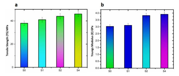
**Figure 6.** Mechanical properties of pristine PS and PS/Sepiolite composites: (**a**) Tensile Strength (TS) and (**b**) Young's Modulus (E).
