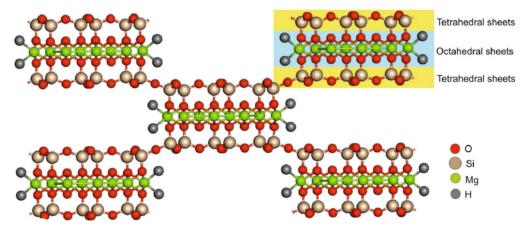
Figure 1. Structure of sepiolite clay. Reprinted/adapted with permission from Ref. [34].
