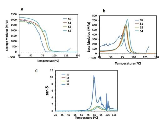
**Figure 7.** Dynamic mechanical analysis of pristine PS and PS/m-sepiolite nanocomposites: (a) Storage Modulus (E''); (b) Loss Modulus (E''); and (c) Damping Factor (tan  $\delta$ ).
