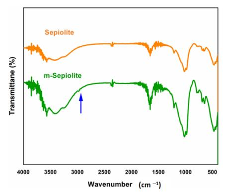
Figure 2. FTIR spectra of pristine sepiolite and modified sepiolite (m-sepiolite) clay.
