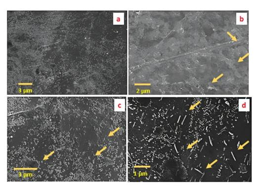
**Figure 5.** SEM images of S0 (pristine PS) in (**a**), S1 (PS/1 wt.% sepiolite) in (**b**), S2 (PS/2 wt.% sepiolite) in (**c**) and S4 (PS/4 wt.% sepiolite) in (**d**).
