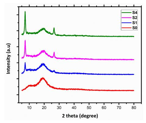
Figure 4. XRD patterns of pristine PS (S0) and PS/m-sepiolite nanocomposites S1, S2 and S4 formulations.
