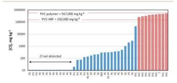
Fig. 1 A selection of plastics analysed by XRF and shown in ascending order of Cl content along with the polymer identified by FTIR (ABS = acrylonitrile butadiene styrene; PE = polyethylene; PP = polypropylene; PS = polystyrene; PU = polyurethane; ? = uncertain and hit quality <70%). Data shown in red and hatched are samples defined as PVC by XRF ([Cl] >150 000 mg kg<sup>-1</sup>). Also annotated is the theoretical Cl content of pure PVC
