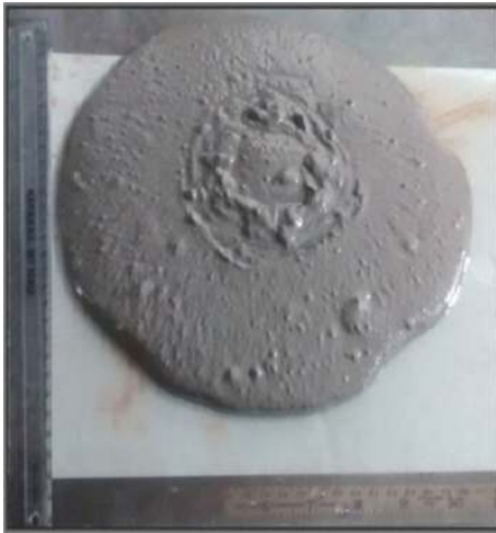
Fig. 4 Flowable mix for measuring spread diameter
