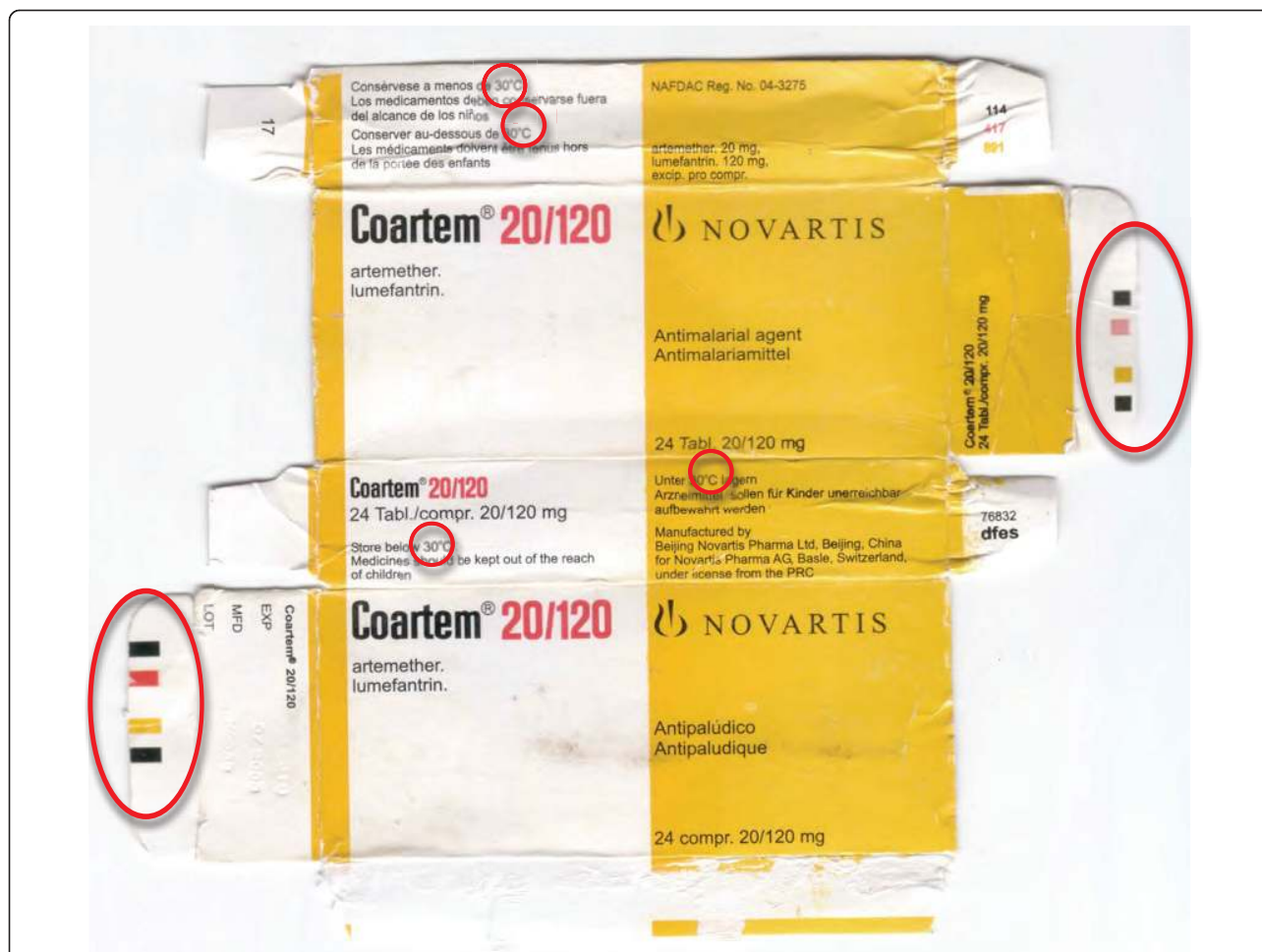
Figure 18 Counterfeit 'Coartem' labelled as made by 'Beijing Novartis Pharma Ltd, Beijing, China for Novartis Pharma AG, Basle, Switzerland' (Gh 09/02). Differences from genuine sample (Figure 16) in red circles.
