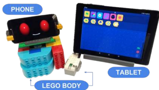
Figure 1: PopBot Components. The social robot is made of a smartphone, LEGO blocks, motors, and sensors. The blocks-based programming interface resides on a tablet.
