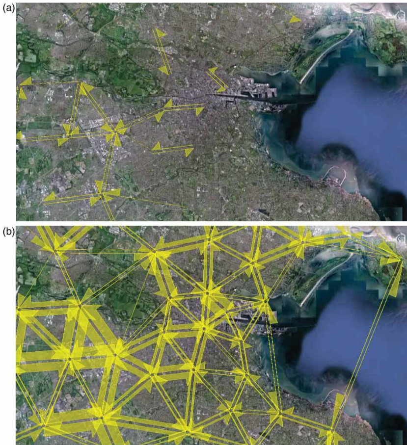
Figure 4: Dublin city regional transition flows in time periods of (a) low, and (b) high intensity, where the width of the connecting arrow corresponds to directional transition intensity. Note connecting arrows with very low intensity have been removed for visual clarity.
