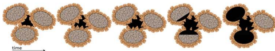
Figure 16. Schematic of the evolution in calcite cemented ooid grainstone porosity during the acidic brine injection- pore volume is shown in black color.
