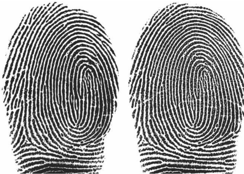
Fig. 11. Two impressions of the same finger at 1,000 ppi. It is observed here that ridge contours are more reliable Level 3 features, compared to pores.
