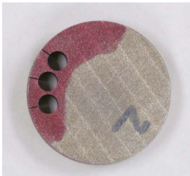
Fig. 1. Sample 3-2, showing where the 5 mm cylinders were cut out via electric discharge machining.
