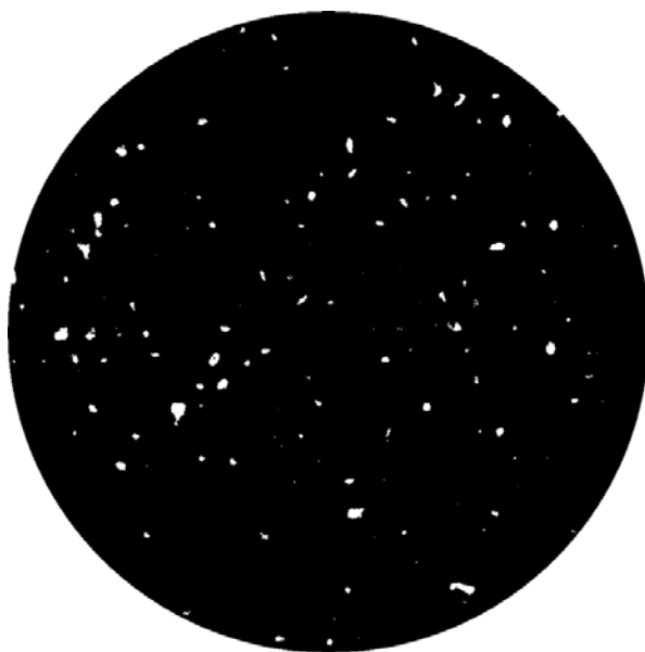
Fig. 7. Same as Fig. 6 but thresholded into solid (black) and pores (white).
