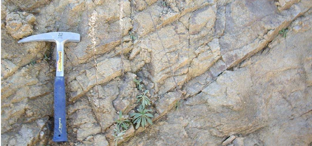
Figure 4. Secondary porosity in the form of parallel joints in fractured Lanseria Gneiss (Johannesburg Dome Granite) from Midrand (Gauteng Province, South Africa); note the varying apertures.
