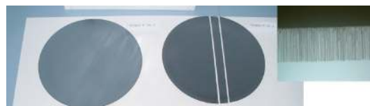
FIGURE 2: First electrochemically etched 200 mm p -type wafers (inset: macropores in organic electrolyte; the most demanding etching process).
