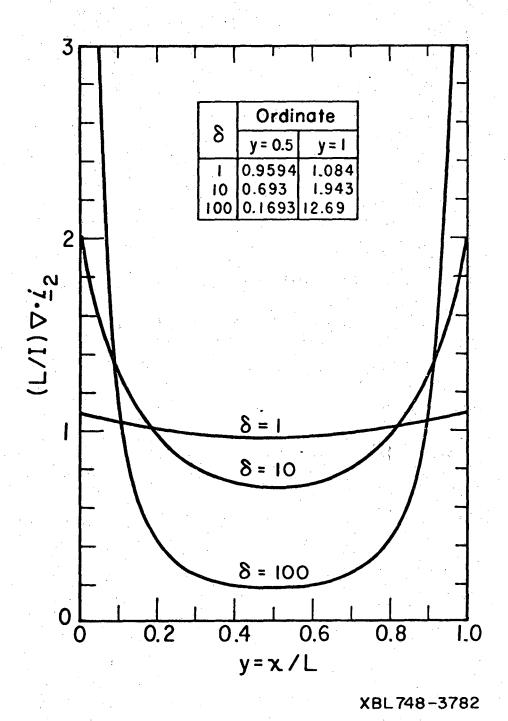
Figure 1. Reduced current distributions for Tafel polarization with  $\,\sigma\,=\,\kappa$  .
