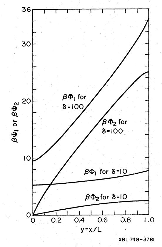
Figure 2. Potential distributions for Tafel polarization with  $\sigma = \kappa$ . Here  $\beta = \alpha_a F/RT$  (or  $-\alpha_c F/RT$  for cathodic currents).
