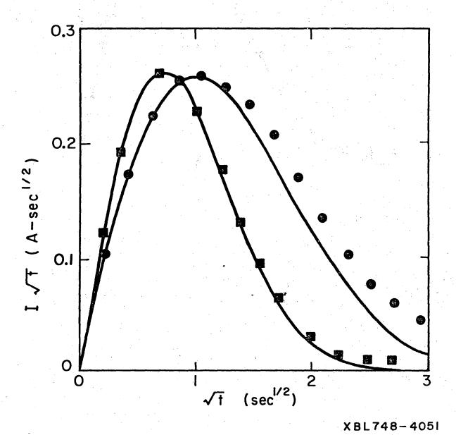
Figure 4. Comparison of experimental and theoretical results for potentiostatic double-layer charging of porous PbO<sub>2</sub> electrodes. Area = 241 cm<sup>2</sup>, L = 0.095 cm, temperature = 28°C.
