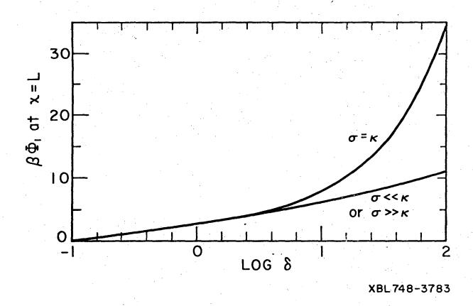
Figure 3. Potential of the metal backing plate as it depends on  $\delta$  . Here  $\beta=\alpha_{f}/RT$  (or  $-\alpha_{c}/RT$  for cathodic currents).
