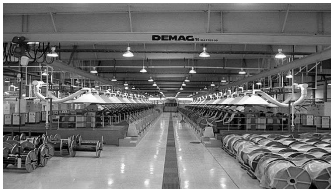
Fig. 11. Nickel foam production unit at the Inco Advanced Technology Materials, Dalian, China (Courtesy of V. Paserin).
