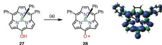
Fig. 10 Synthesis of the subporphyrin meso -oxy radical 28 (isovalue = 0.001). (a) 800 equiv. PbO_2 , CH_2Cl_2 , rt, quant.
