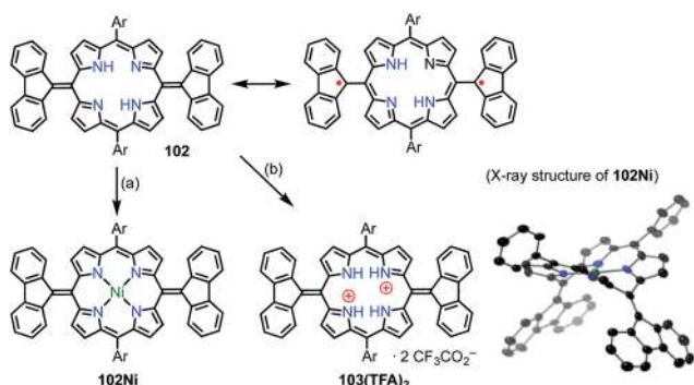
Fig. 33 5,15-Bis(9-fluorenyl)porphyrins and X-ray crystal structure of 102Ni . (a) 10 equiv. Ni(OAc) 2 ·4H 2 O, toluene, 120 °C, 5 h, quant.; (b) 2 equiv. CF 3 CO 2 H, CH 2 Cl 2 , <10 min, quant. Ar = 3,5-di- tert -butylphenyl. Hydrogen atoms and tert -butyl groups in the crystal structure of 102Ni are omitted for clarity.
