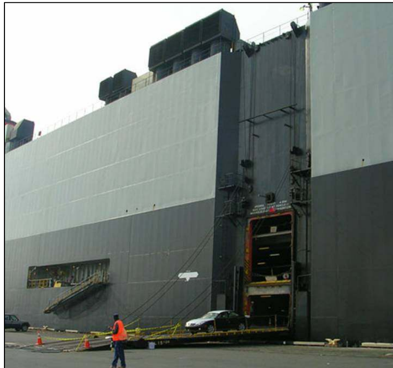
Figure 6.3 Roll-On Roll-Off (RoRo) ship. nd. Photograph. The process of offloading passenger vehicle cargo from a ship is shown.
