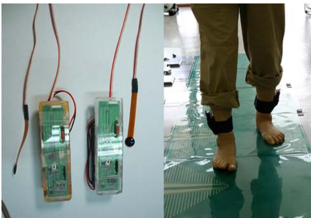
Fig. 2 Photos of the portable activity monitoring system and foot switches
