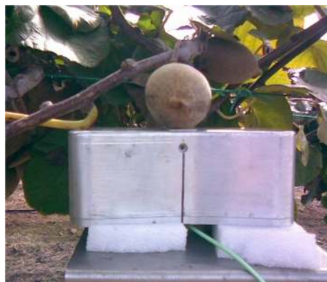
Fig. 9 NMR measurements in field on entire kiwifruits attached to the plant (Reproduced with permission from [49])
