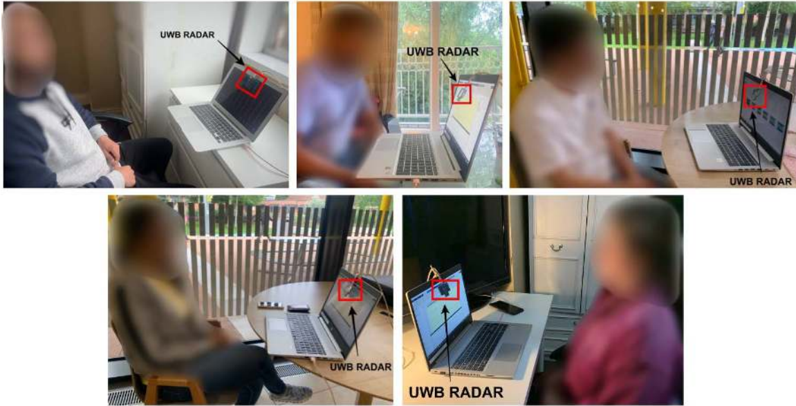
Fig. 5. Respiratory data acquisition in a static environment through diverse individuals.
