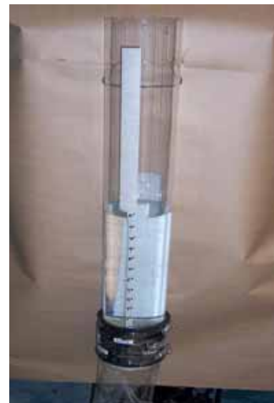
Fig. (1). Permeameter for PCPC.
