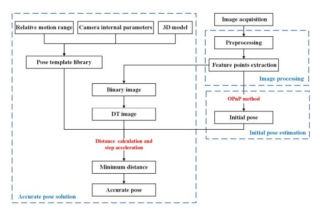
Figure 1. Flow diagram of the pose estimation method.
