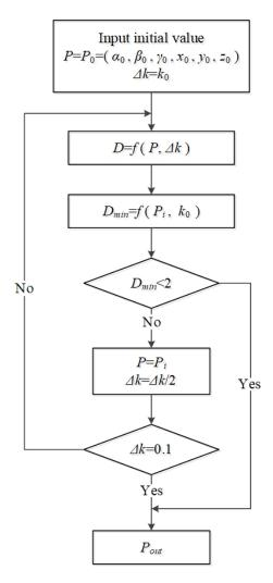
**Figure 5.** The structural block diagram of the step acceleration process.
