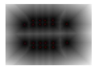
**Figure 4.** DT image. The distances are gray-level coded: the larger the distance the lighter the tone. The red cross are the feature points of the cutter holder.
