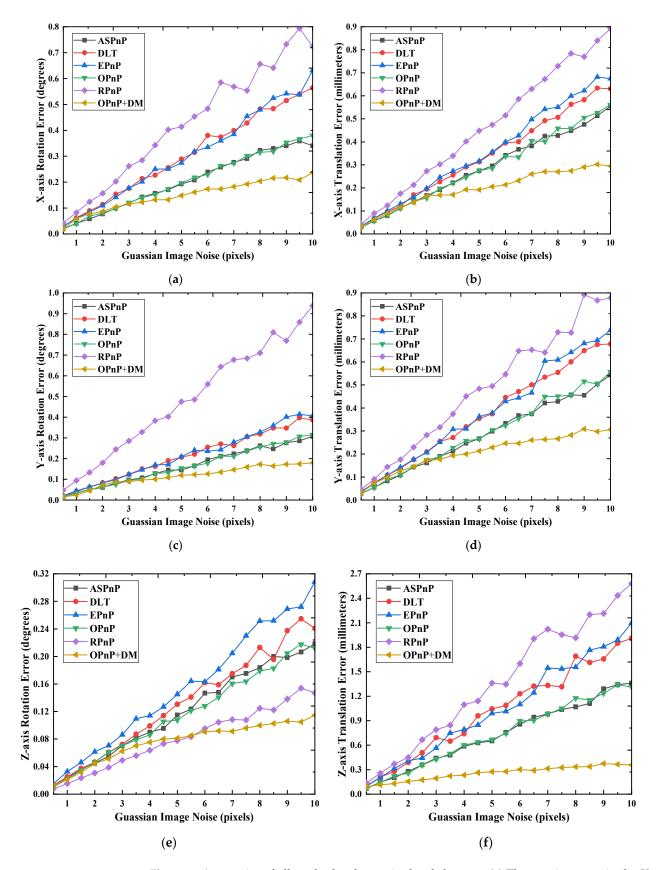
**Figure 6.** Accuracies of all methods when noise level changes. (a) The rotation error in the *X*-axis direction; (b) The movement error in the *X*-axis direction; (c) The rotation error in the *Y*-axis direction; (d) The movement error in the *Y*-axis direction; (e) The rotation error in the *Z*-axis direction; (f) The movement error in the *Z*-axis direction.
