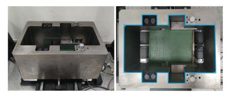
**Figure 2.** The physical photo of the cutter holder. The blue curve on the surface of the cutter holder on the right is its inside contour.
