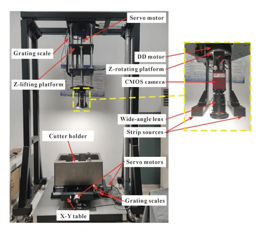
Figure 7. Visual system and four-axis motion platform.
