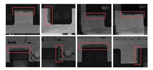
**Figure 9.** Partial images of the contaminated parts of the cutter holder. The red boxes show the various contamination conditions of the cutter holder.
