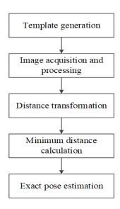
Figure 3. Flowchart of distance matching method.
