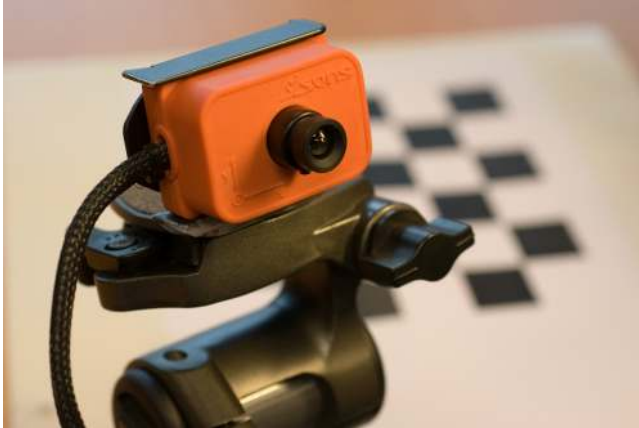
Figure 6.2: The sensor unit is mounted on a tripod for calibration. The background shows the camera calibration pattern that has been used in the experiments.
