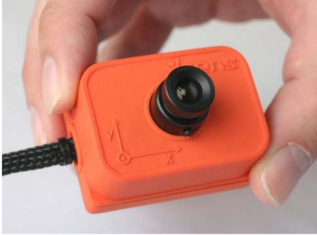
Figure 2.1: A prototype of the MATRIS project, integrating a camera and an IMU in a single housing. It provides a hardware synchronized stream of video and inertial data.
