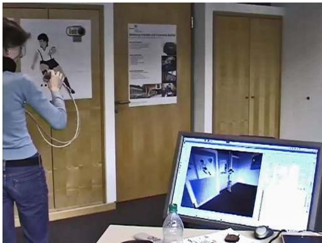
Figure 7.1: The sensor unit is tracked in a large room. The monitor shows the live camera image augmented with a virtual character.
