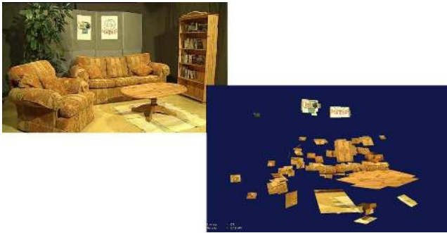
Figure 2.2: An example of a scene model consisting of planar patches (lower right) and the actual scene that is modeled (upper left).
