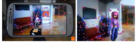
Fig. 11. AR system that considers first an off-line SLAM approach followed by an on-line PnP [81]. The reduced computational complexity allows an implementation on a smartphone (a video is available here ).
