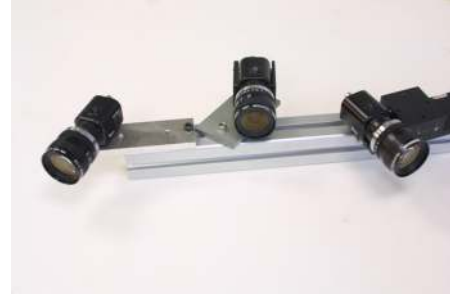
Fig 2. The MCS used in our experiment that consists of three CCD cameras.
