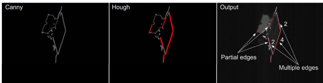
Figure 3 Steps of image processing process: Canny edge detector (left), Hough transform (middle), and output segments superimposed to original image (right).
