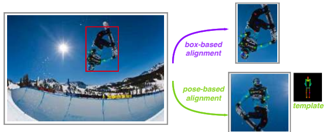
Figure 2: Comparison of box-based alignment and our pose-based alignment ( Affine-Align ). Objects with strange pose are corrected to a standard pose.
