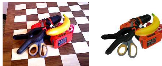
Fig. 6. Left: an example image from the dataset. Right: Textured 3D object models (provided with the YCB dataset) rendered according to the pose annotations for this frame.
