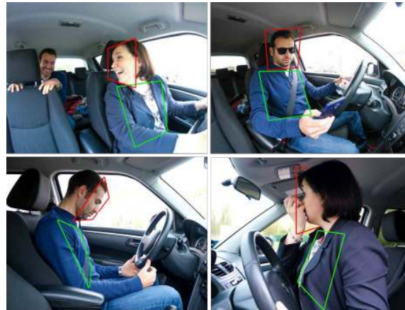
Figure 1. Some real situations in which head and upper-body pose estimation are useful to monitor driver’s attention level: from the top-left, driver is talking with passengers, is playing with smartphone, is falling sleep and is looking at the rear-view mirror.
