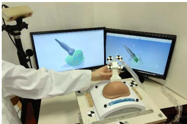
Fig. 1 The FUS system allows to map the real positions of the CIRS breast phantom and the US probe to the 3D Slicer scene (right monitor). Information about probe spatial transformation is communicated to the simulated environment in Unity (left monitor)
