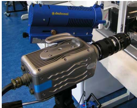
Figure 4.4: High speed camera utilization. (a) Lighting setup. (b) Highspeed camera with the 2x tele-converted portrait lens (55mm micro nikkor) and Dedocool video lamp.
