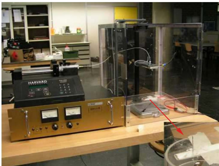
Figure 2.6: Electrospinning test setup
