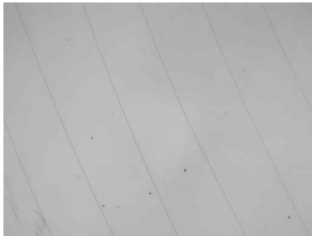
Figure 4.5: Electrospun spirals on a small glass disc with a collecting speed of 8m/s and a spacing of 1mm . The image has been taken on a Zeiss lightmicroscope (type Axioplan 2) using a lens with 1,5x magnification
