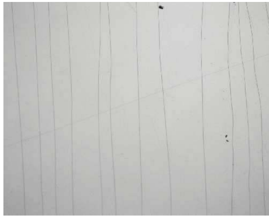
Figure 4.3: Electrospun spirals on a smaller mylar disc with a collecting speed of 8m/s and a (desired) spacing of 0.25mm . The image has been taken on a Zeiss lightmicroscope (type Axioplan 2) using a lens with 2,5x magnification
