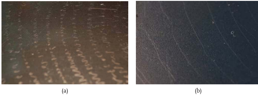
Figure 4.2: Surfaces of spun discs with different collecting speeds. Collecting speeds: (a) 2m/s (b) 8m/s .
