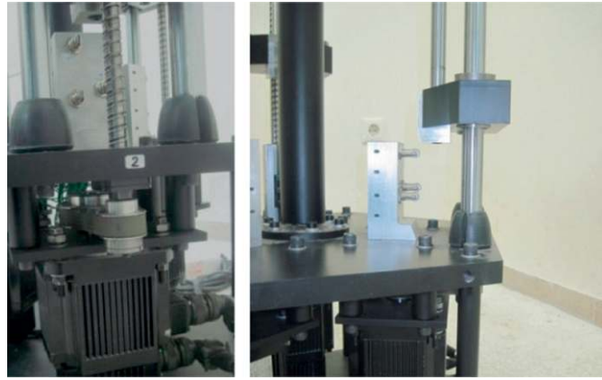
Fig. 5. The i th motor, ball screw and nut assembly.
