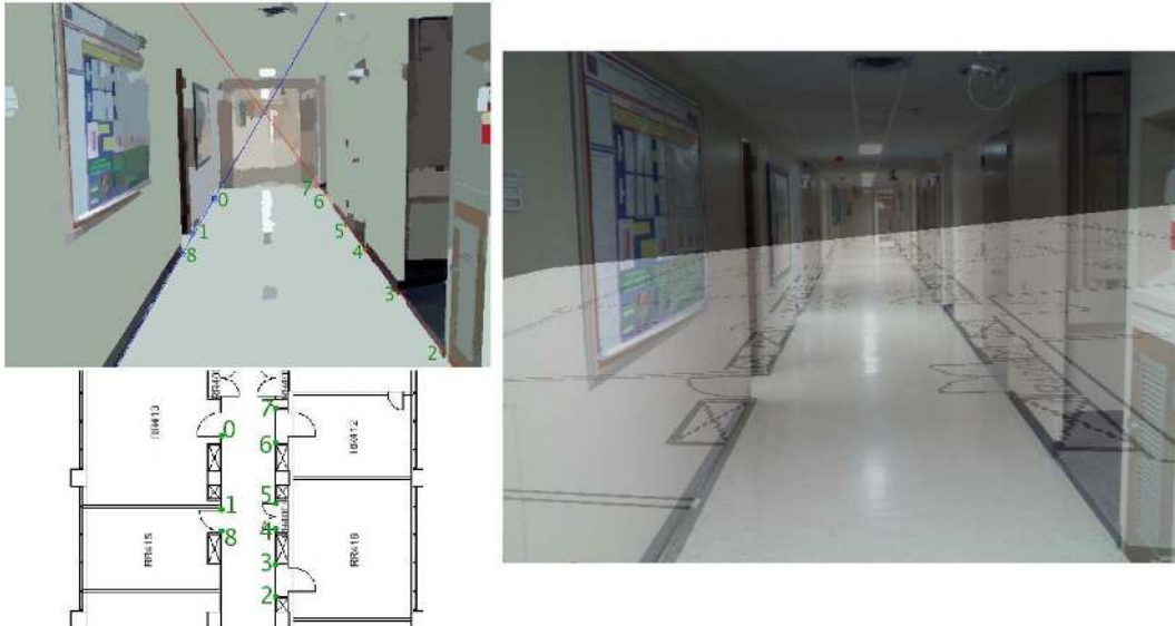
Figure 5: Results of point correspondence algorithm. Upper left: the detected points on the image labeled by number. The detected points of this example required some manual filtering to get a good match. Lower left: the points on the floorplan that were matched to the image, labeled with corresponding numbers. Right: floorplan warped into the image space and overlaid on top of the original image. This example has 9 image points and 19 map points and completes matching in about 2 seconds.
