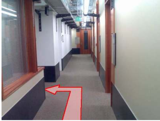
Figure 6: This shows an arrow overlaid to match the perspective of the floor. The calculated homography was used to place the arrow.
