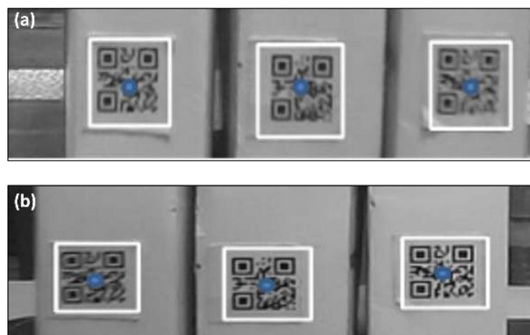
Figure 14. A set of QR code images acquired by the robot binocular vision system. (a) QR images obtained by left-hand side camera. (b) QR images acquired by the right-hand side camera.
