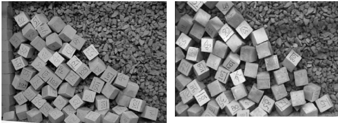
drop height 2.5 D_{\text{cube}} , placing density 72%
