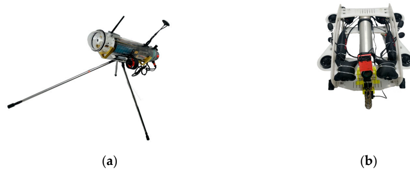
Figure 7. Sea trial experimental equipment. (a) Autonomous tracking buoy; (b) remotely operated vehicle (ROV).
