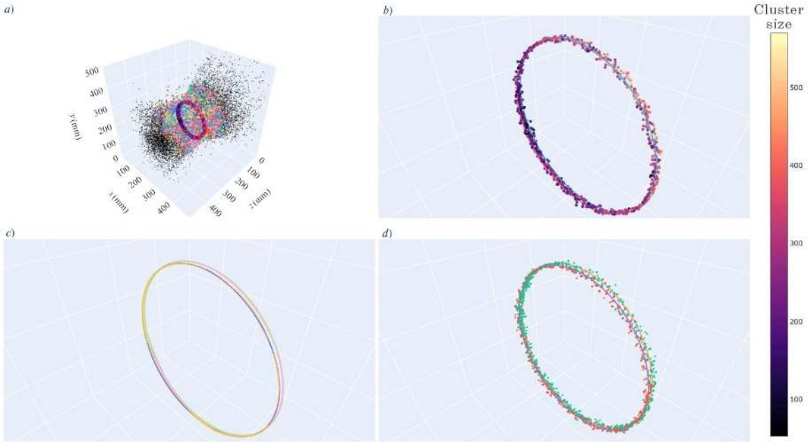
FIG. 5. Tracking two particles rotating at 42 RPM, each describing one full circle. Plot a) depicts all the cutpoints after one pass of clustering using PEPT-ML: in colour are cutpoints which were clustered; in black are the cutpoints deemed as noise. Plot b) shows the centres of the clusters from the previous plot: the number of points in the cluster (“cluster size”) is colour-coded from purple to yellow. Here, purple represents a smaller cluster size, corresponding to less tracer activity, while yellow represents a larger cluster size, corresponding to more tracer activity. Plot c) depicts the cluster centres after the second pass of clustering using PEPT-ML (see section II C), after trajectory separation has been applied in the post-processing step (see section II D). Plot d) depicts the trajectories found using the Birmingham algorithm. In both images c) and d), the solid lines shown correspond to the ‘real’, analytically-determined circular path followed by the tracers.
