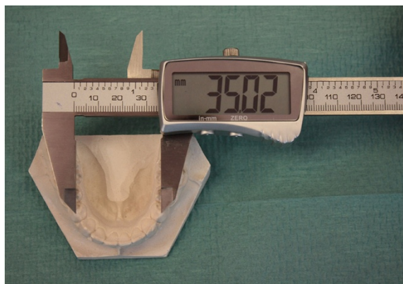
Figure 2 Hand held digital caliper with accuracy of 0.01mm used for measuring distances of specified points.
