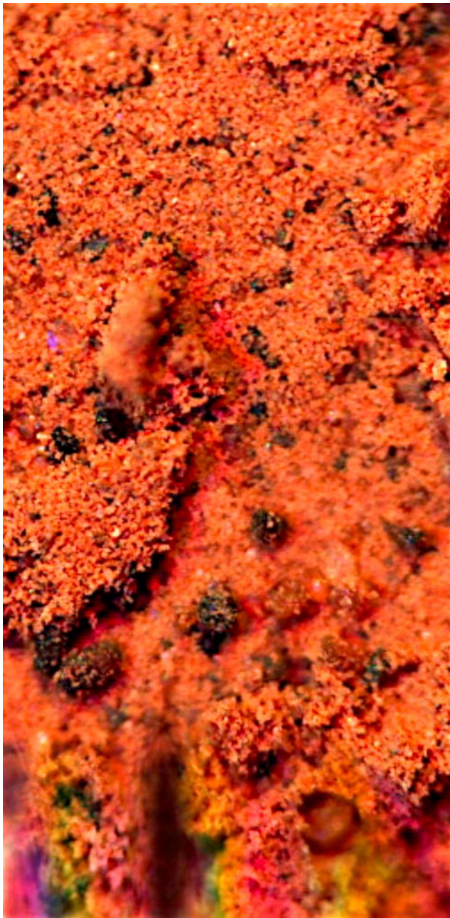
Figure 5. Possible evidence of salt particles in a full color OM image of a sample of soil from the Phoenix landing site. The image is 1 mm wide. A substantial fraction of the ubiquitous whitish particles are probably salts. This idea is consistent with measurements by the Phoenix TEGA and WCL.
