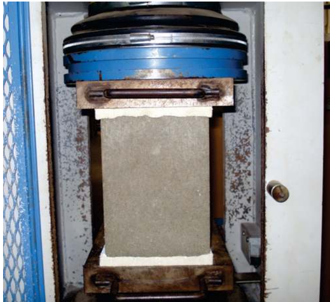
Figure 5 – Test of resistance to compression of the blocks
