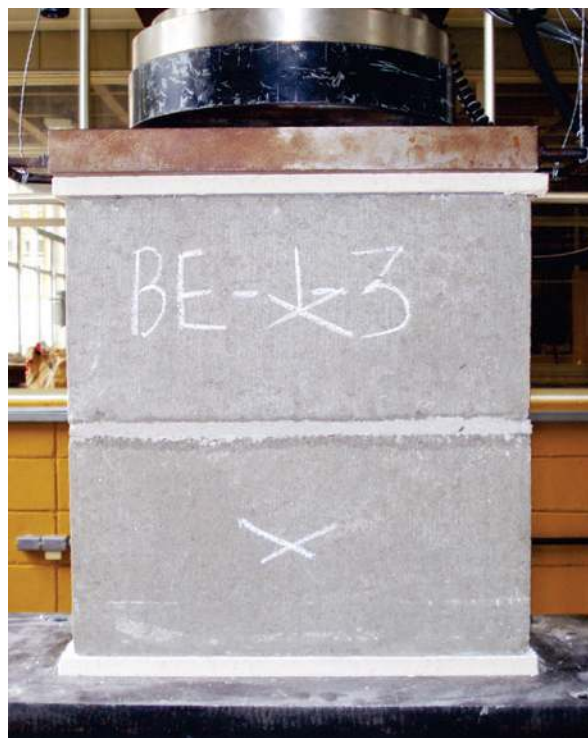
Figure 6 – Test of resistance to compression of the prisms and small walls
