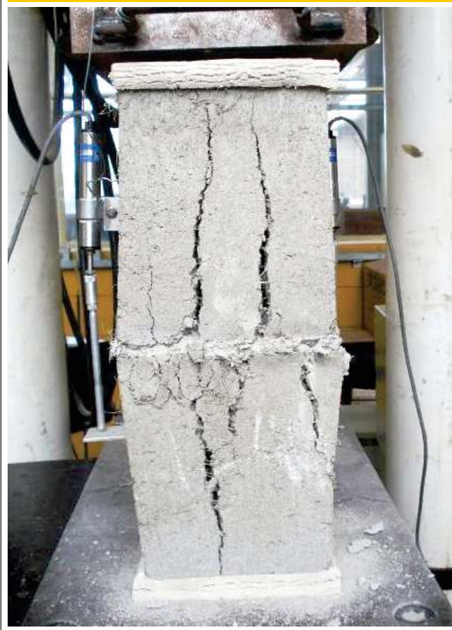
Figure 12 – Ductile break of the prisms with the added fiber
