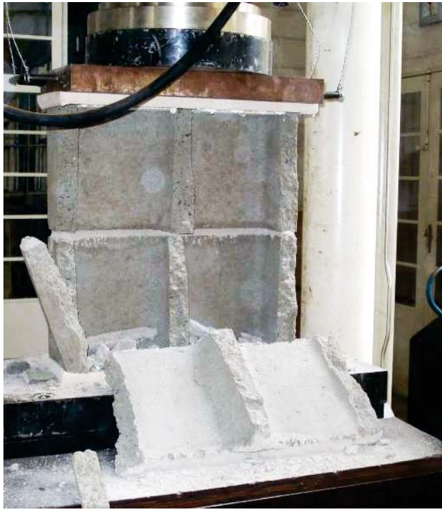
Figure 13 – Fragile break of the prisms without the added fiber
