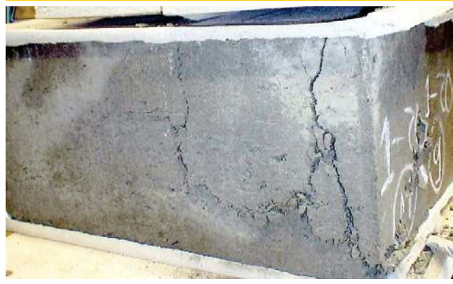
Figure 11 – Ductile break for the blocks with the added fiber
