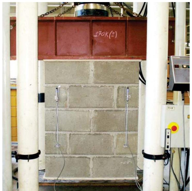
Figure 6 – Test of resistance to compression of the prisms and small walls
