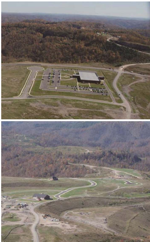
Fig. 10 Commercial and residential post-mining land uses must ensure stable land surfaces and no mass movement of materials for structures to be safe
