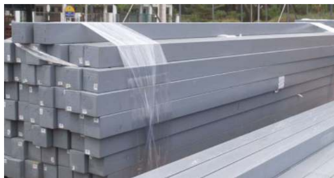
FIGURE 5: Cross arm beams in stockpiles after pultrusion for distribution.
