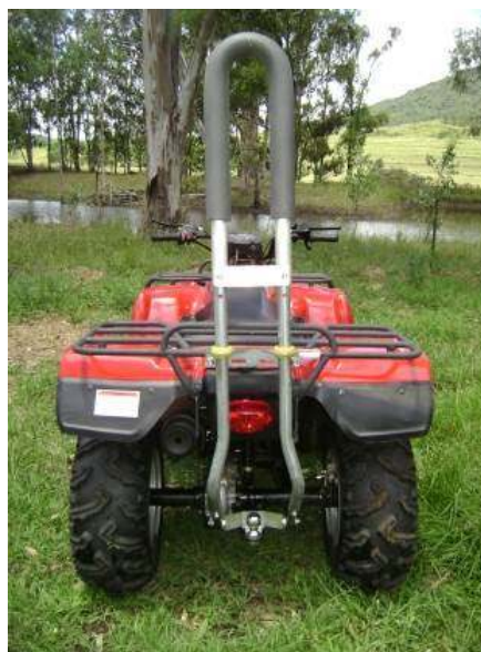
Figure 2. A Quadbar™ attached to the rear of an all-terrain vehicle.
