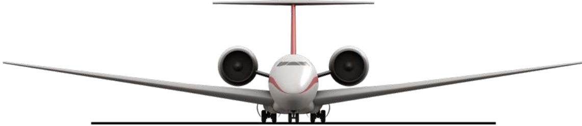
Figure 7. NASA N+2 technology MFN301-GTF-PG aircraft model, front view, with nose fairing portion of the pod retracted.
