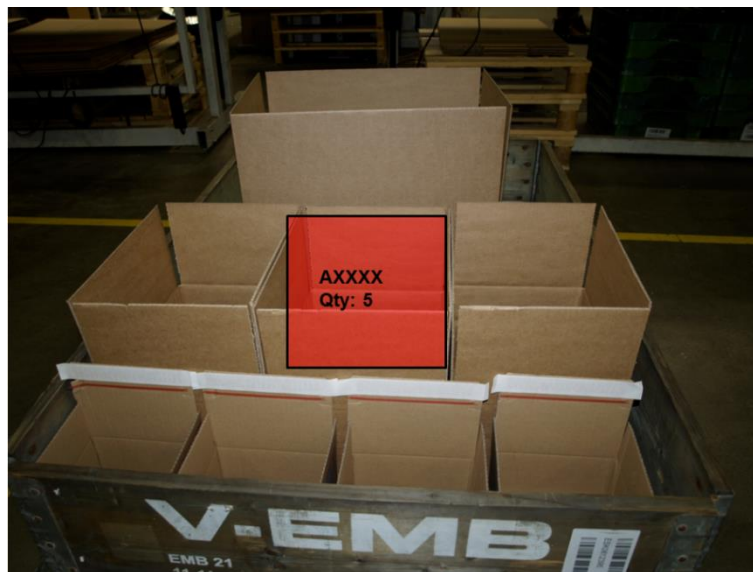
Figure 5.22: Interactive two dimensional illustration of how to place the part during picking
